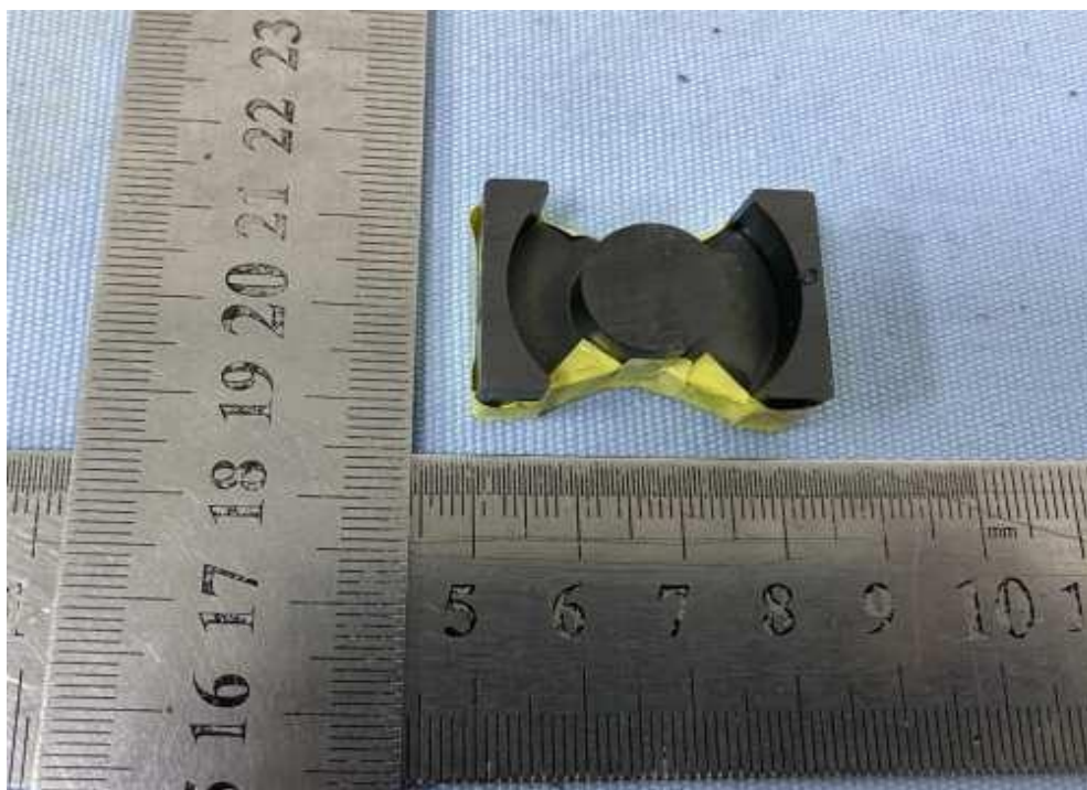
Figure 16. Internal view of transformer
