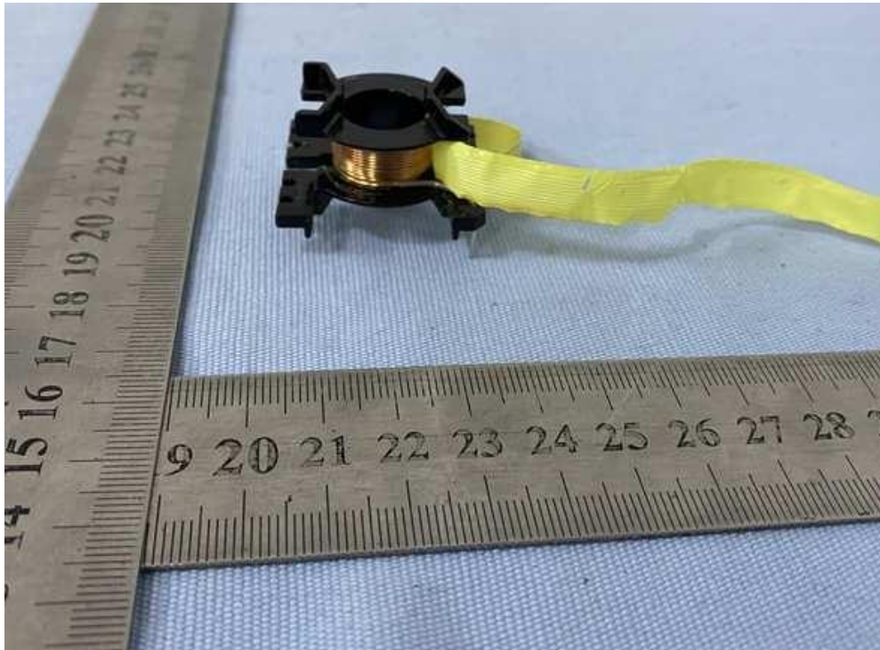
Figure 25. Internal view of transformer
