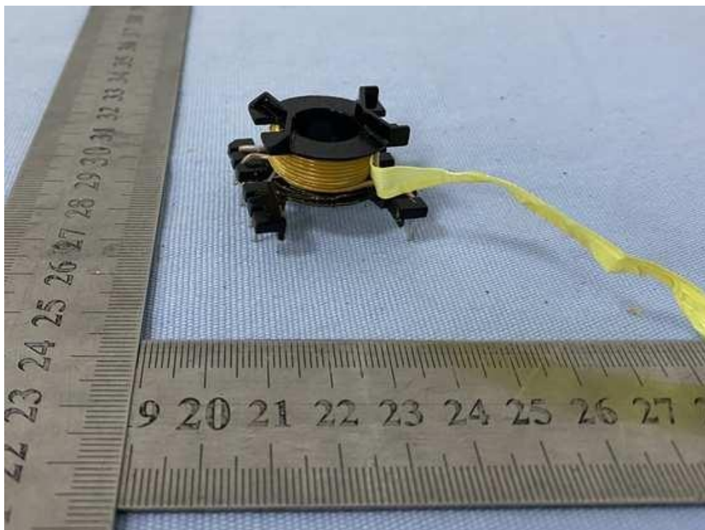
Figure 23. Internal view of transformer
